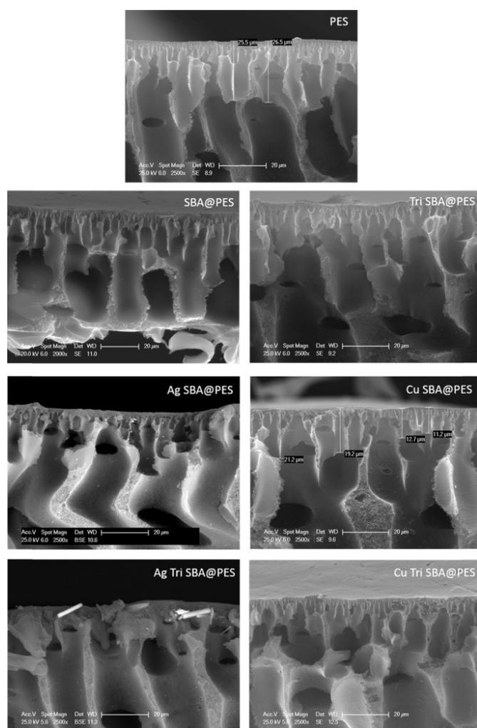
**Figure 1.** Cross-sectional SEM micrographs of membranes manufactured in this investigation.
