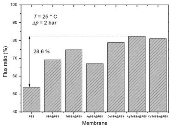
**Figure 4.** Evaluation of irreversible fouling of membranes in terms of pure water flux decline after filtration of 1 g/L BSA solution.
