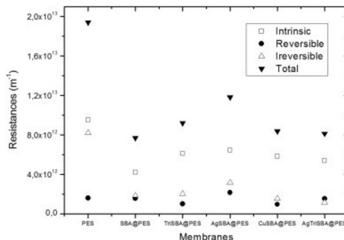
**Figure 5.** Membrane fouling resistances determined from filtration experiments.
