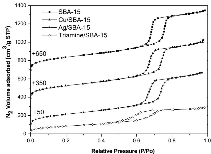
Fig. S2. Nitrogen adsorption-desorption isotherms of SBA-15 and functionalized materials.
