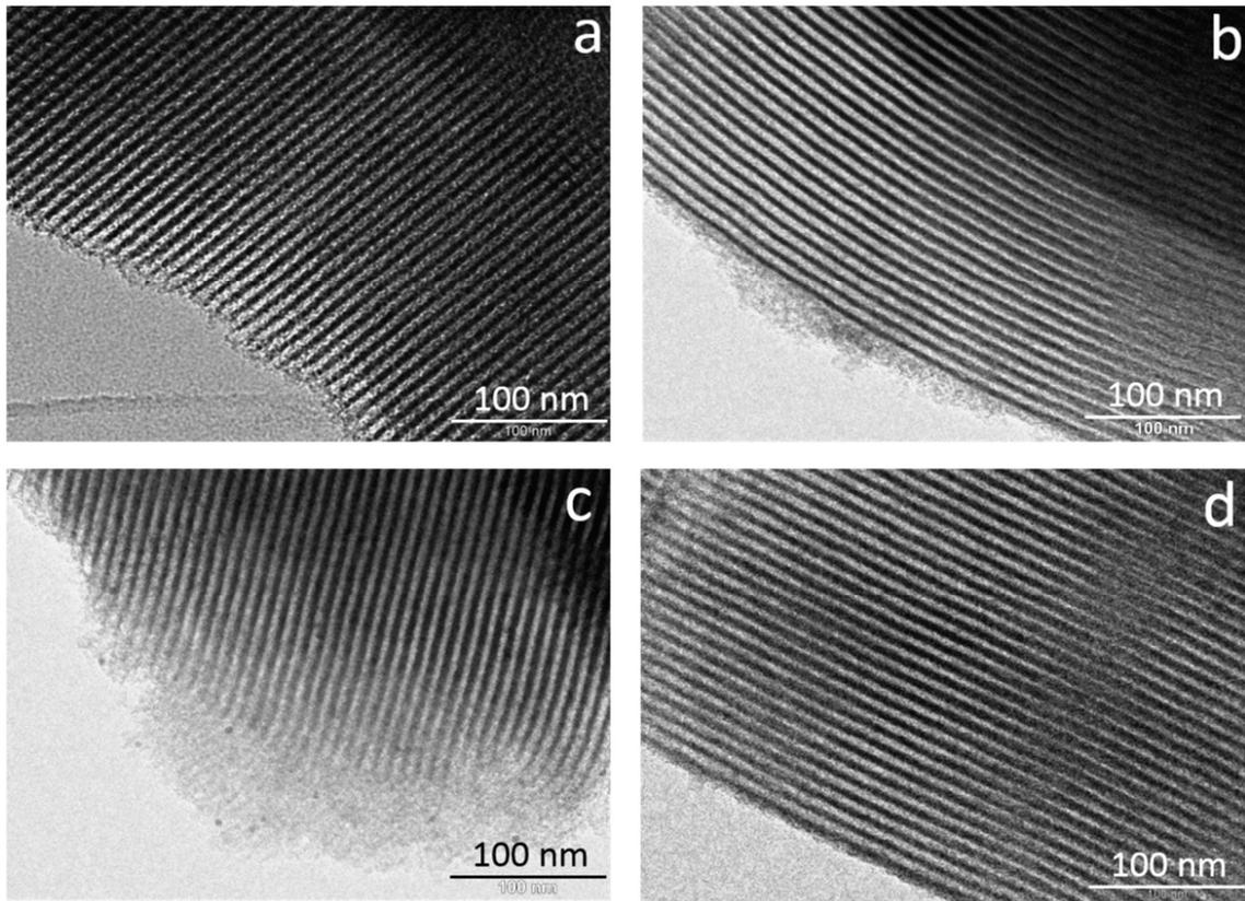
**Fig. S3.** TEM micrographs of (a) SBA-15, (b) Cu/SBA-15, (c) Ag/SBA-15 and (d) Triamine/SBA-15.
