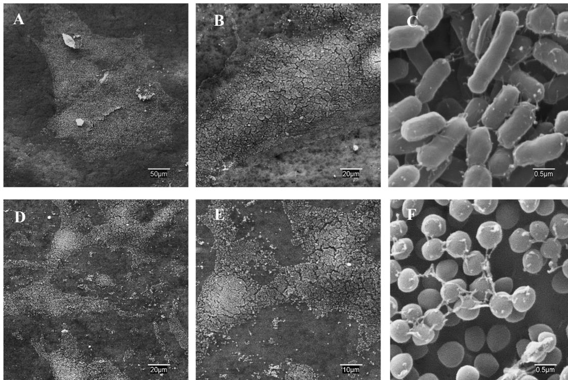
**Fig. S6.** Microbial colonization of TriSBA@PES membranes exposed to *E. coli* (A-B-C) and *S. aureus* (D-E-F) for 20 h at 36 °C. The different magnifications show irregular colonization patterns and biofilm formation.
