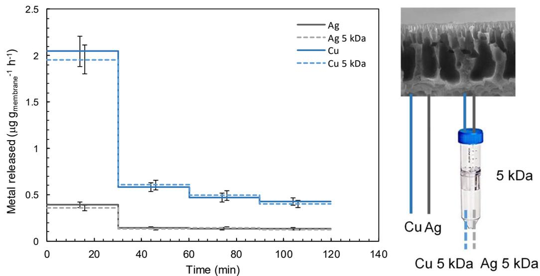
**Figure S9.** ICP-MS analyses of permeate from AgSBA@PES and CuSBA@PES before (solid lines) and after (dashed lines) 5 kDa ultrafiltration of membrane permeate. Error bars show no significant differences for silver (in grey) and copper (in blue).
