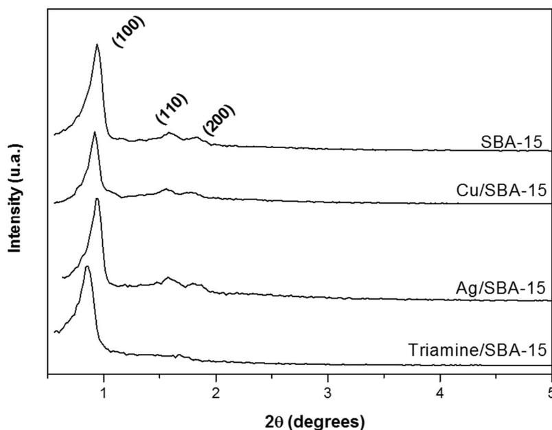
Fig. S1. Low angle XRD patterns of pure SBA-15 and functionalized materials.
