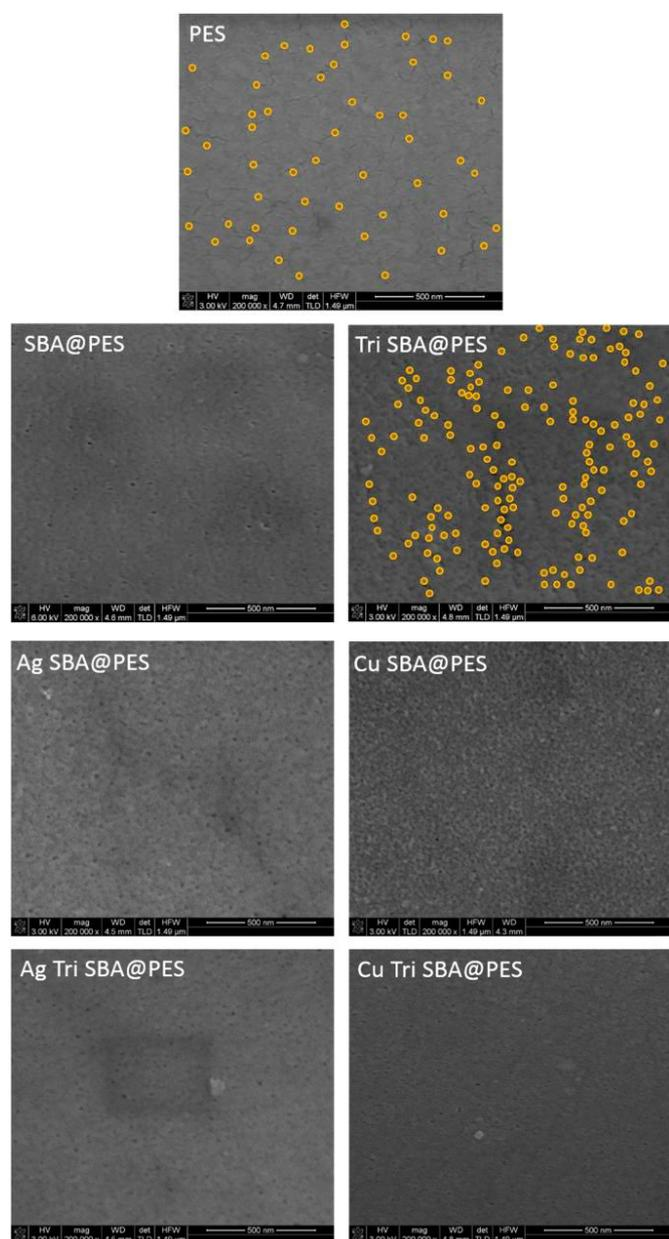
**Figure 2.** FEG-SEM images of manufactured membranes surfaces. Yellow circles have been drawn around pores to facilitate visual interpretation.
