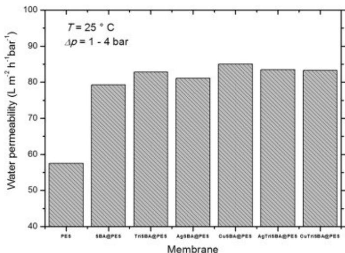
**Figure 3.** Pure water permeability for neat PES and hybrid membranes.
