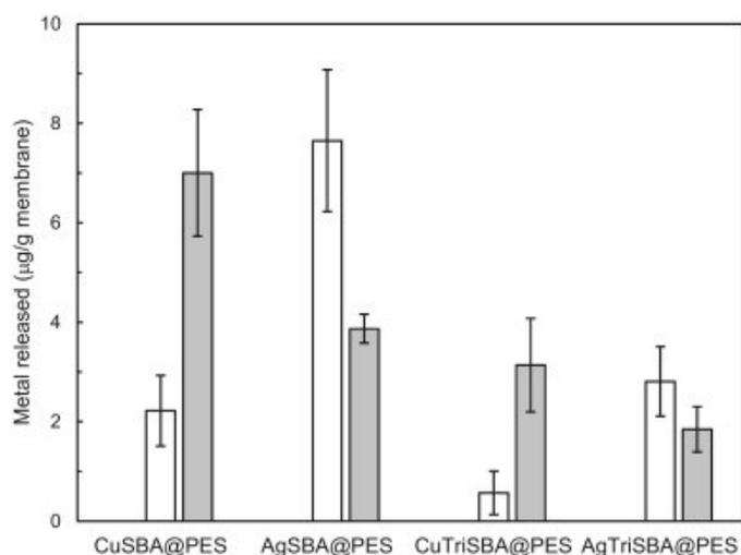
**Figure 8.** Metal released per unit mass of membrane after 20 h in contact with water (empty bars) or NB 1/500 culture medium (grey bars).
