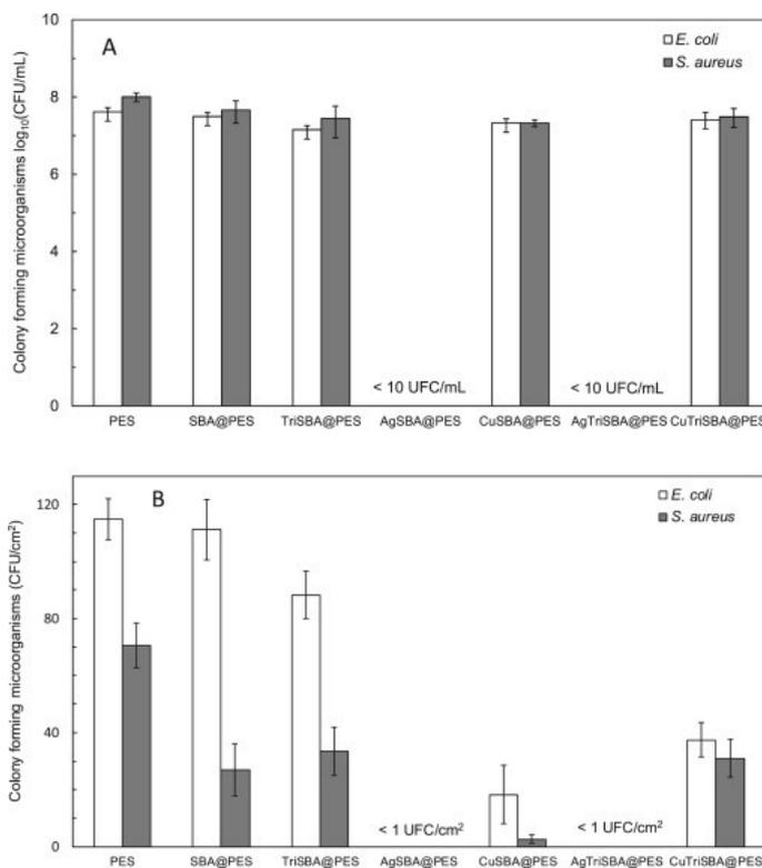
**Figure 6.** Microbial growth for bacterial cultures exposed to membranes (A) and culturable bacteria detached from membranes after incubation (B) at 36 °C, 20 h.
