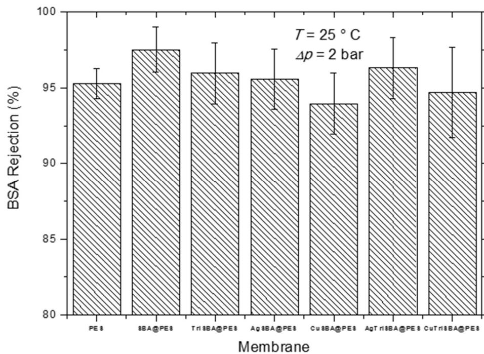
**Fig. S4.** BSA rejection of manufactured membranes for 1 g/L BSA aqueous solutions at 2 bar TMP.
